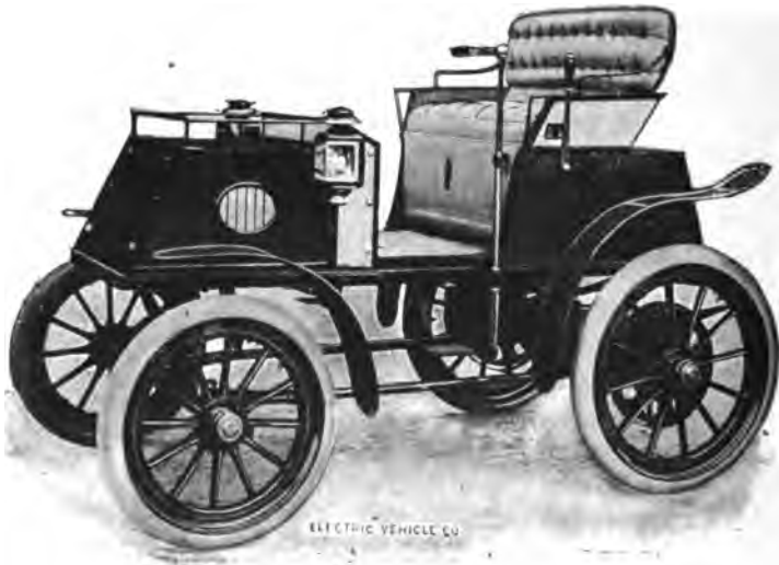
FIG. 438a.—“Columbia” Electric Runabout. This carriage, weighing about 1,900 pounds, has a traveling radius of about forty miles per full charge of battery, and a maximum speed of thirteen miles per hour.
